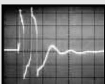
*Oscilloscope reveals high frequency transients coming from the output of a conventional power protection product. These transients can pit, scar and corrode delicate microprocessor circuitry, causing components to run hot, run unreliably and eventually fail.*
